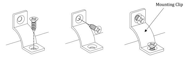
2. Position the Trace fixture inside of the mounting clips to the desired position and fully tighten the screws to secure the Trace fixture.
